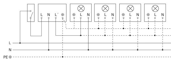
**Connection using two-circuit switch for manual and automatic operation**
