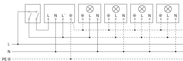
**Circuit diagram Connection via a changeover switch for continuous and automatic operation**
